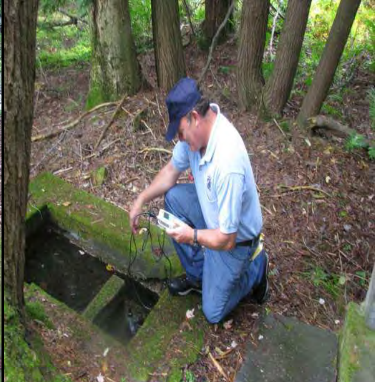
Contaminated shallow groundwater system/spring from spills and inadequate of containment of buried drill cuttings, Alex Branch (HQ), Clearfield County
