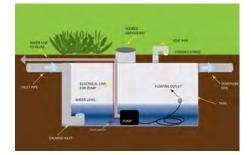
A cistern serves a similar function to a rain barrel but is larger and often used on farms or large estates to capture and store water. A cistern can be an above ground or below ground tank.
