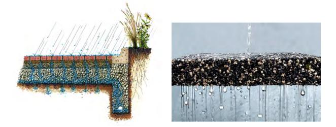
Most concrete and asphalt paving is impervious meaning that it does not allow water to pass through. There are a number of paving options now that allow water to pass through and they are collectively referred to as pervious paving.
