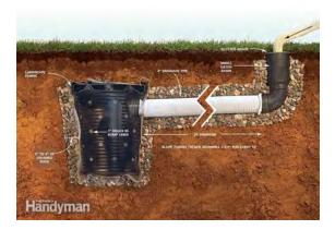
A dry well is a small, excavated pit filled with stone or gravel that temporarily stores stormwater runoff until it soaks into the surrounding soil. A dry well serves the same function as a rain garden but is underground. You can purchase a prefabricated dry well or build one with stone and gravel.
