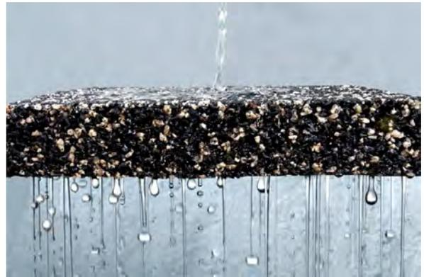
Most concrete and asphalt paving is impervious meaning that it does not allow water to pass through. There are a number of paving options now that allow water to pass through and they are collectively referred to as pervious paving.
